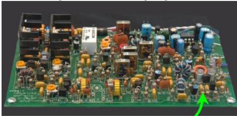
Measure VFO Frequency Here (top of R-27)
